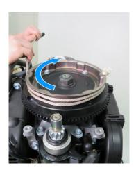
8. Wind the emergency starter rope clockwise around the fly wheel along the groove in the flywheel.
