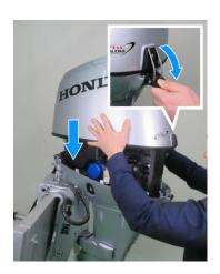
10. Leave the flywheel cover off and install the engine cover.
