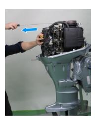
13. Pull the emergency starter rope several times to lubricate the inside of the cylinder. Then remove the emergency starter rope.
