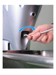
After draining the oil, install the drain bolt and new sealing washer, and tighten the bolt securely. Install the drain bolt cover.
