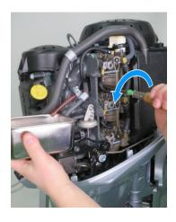
Drain the fuel from all the carburetor. Make sure the drain screws are tightened after draining.
