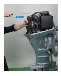
9. Pull the starter rope lightly until resistance is felt, then pull firmly to start the engine.
