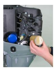
12. Pour a teaspoon of engine oil into all the spark plug holes.
