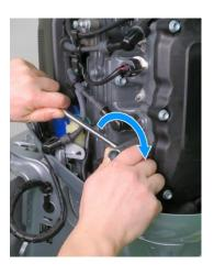
14. Carefully install the spark plugs by hand to avoid crossthreading. Tighten 1/8—1/4 turn after the spark plug seats. Install the ACG cover.
