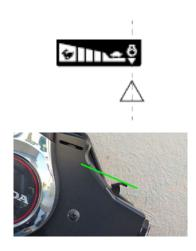
6. Tiller handle type: Align the "start" mark on the throttle grip with the projected end of the "▲" mark on the tiller handle.
