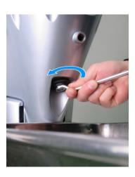
8. Place a suitable container under the oil drain guide, remove the drain bolt cover, engine oil drain bolt and washer. Drain the engine oil until the flow of old oil reduces to a trickle.
