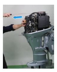
6. Remove the flywheel cover. Wind the emergency starter rope (Refer to the Emergency starting procedure.) Drain the water from the cylinder by pulling the emergency starter rope several times.
