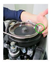
7. Set the knotted end of the emergency starter rope in the notch in the flywheel.
