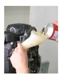
10. Refill to the upper level mark on the oil level dipstick with the recommended oil. Do not overfill. Too much engine oil may adversely affect the engine.
