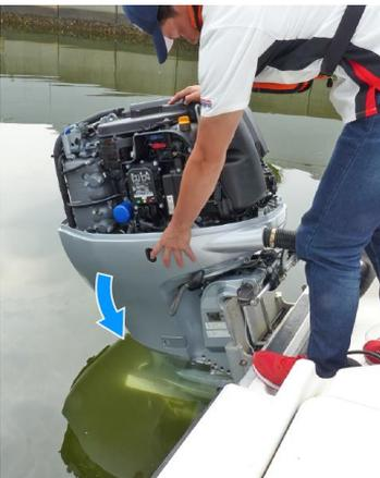
8. Tilt the outboard motor down.
