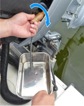
6. After draining, tighten the drain screw.
