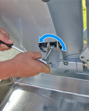
10. Place a suitable container under the oil drain guide, Set the drain plug cover under the guide. remove the engine oil drain bolt and washer. Drain the engine oil until the flow of old oil reduces to a trickle.
