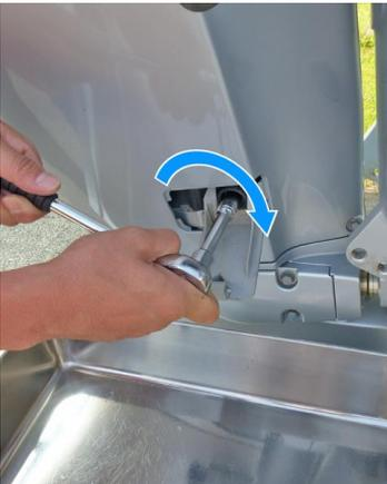
11. After draining the oil, install the drain bolt and new sealing washer, and tighten the bolt securely.
