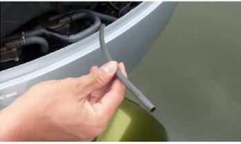
3. Set the end of the tube toward the outside of the engine undercase. Draining the fuel becomes easier when the front end of the drain tube is as low as possible.
