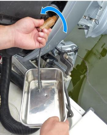
3. Set the end of the tube toward the outside of the engine undercase. Draining the fuel becomes easier when the front end of the drain tube is as low as possible.
