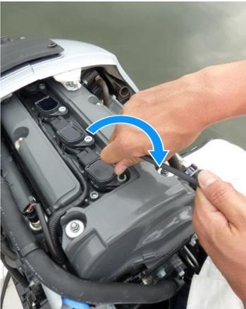
16. Carefully install the spark plugs by hand to avoid cross-threading. Tighten  $1/8$ – $1/4$  turn after the spark plug seats. Install the ACG cover.
