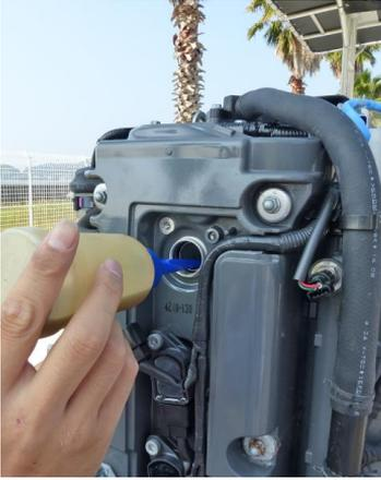
15. Pour a teaspoon of engine oil into all the spark plug holes to lubricate the inside of the cylinders.
