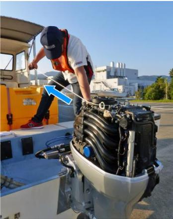
16. Pull the emergency starter rope several times to lubricate the inside of the cylinder. Then remove the emergency starter rope. See “If the starting system does not operate” to set the emergency starter rope.
