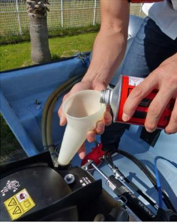
12. Refill to the upper level mark on the oil level dipstick with the recommended oil. Do not overfill. Too much engine oil may adversely affect the engine.
