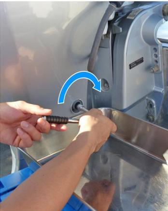
11. After draining the oil, install the drain bolt and new sealing washer, and tighten the bolt securely.
