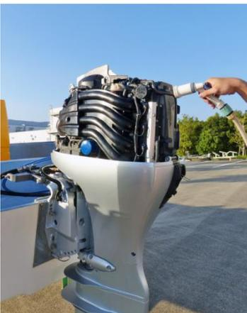
2. Rinse the outboard motor with fresh water to remove salt water, sand, mud, etc.
