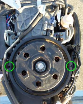
8. Turn the AC generator rotor clockwise so that the cutouts are on the right and left sides of the AC generator rotor as shown.
