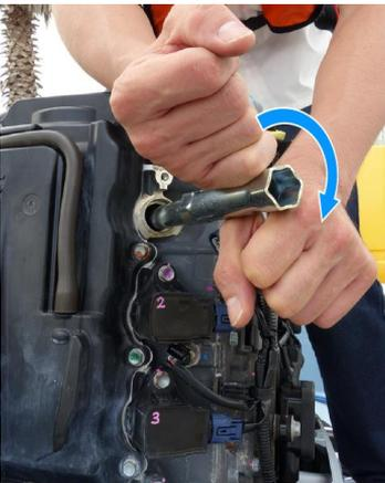
17. Carefully install the spark plugs by hand to avoid cross-threading. Tighten  $1/8$ – $1/4$  turn after the spark plug seats. Install the ACG cover.
