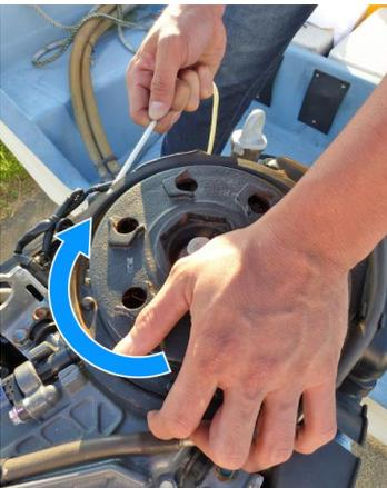
10. Wind the emergency starter rope clockwise around the fly wheel along the groove in the AC generator rotor.
