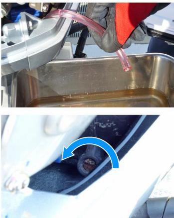
5. Loosen the vapor separator drain screw. Drain the petrol into the drain pan as it flows out of the drain tube.
