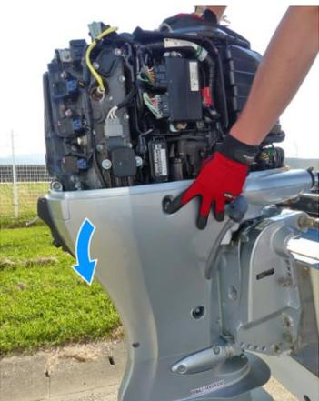
8. Tilt the outboard motor down.
