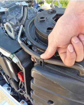
5. Secure the breather tube to the clamp of the silencer case.
