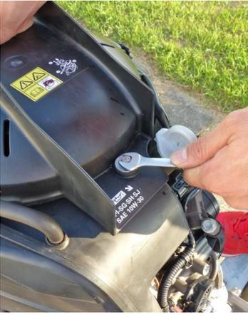
4. Remove the flange bolt and washer, then remove the ACG cover.
