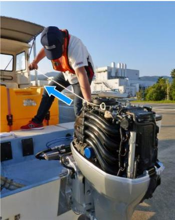
13. Pull the starter rope lightly until resistance is felt, then pull firmly.
