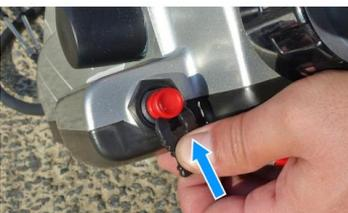
11. Insert the emergency clip into the emergency stop switch. Attach the other end of the emergency stop switch lanyard securely to the operator.
