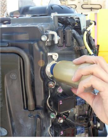
15. Pour a teaspoon of engine oil into all the spark plug holes.
