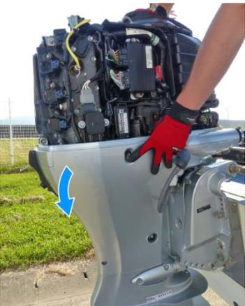
8. Tilt the outboard motor down.
