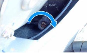
6. After draining, tighten the drain screw.
