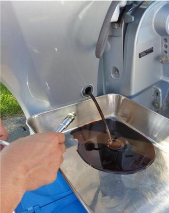
10. Place a suitable container under the oil drain guide, remove the engine oil drain bolt and washer. Drain the engine oil until the flow of old oil reduces to a trickle.
