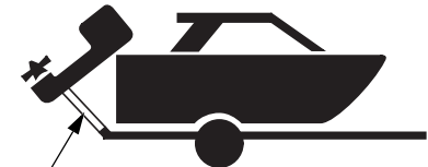
OUTBOARD MOTOR SUPPORT BAR (commercially available)
