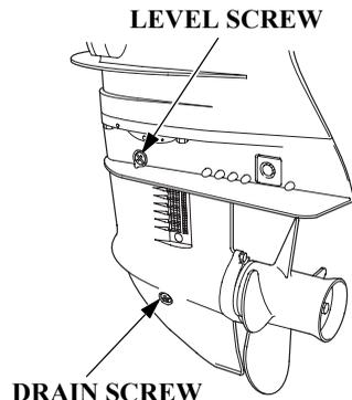
1. Position the outboard motor vertically.
