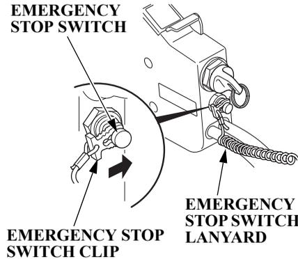
The emergency stop switch lanyard is provided to stop the engine immediately when the operator falls overboard or away from the outboard motor.
