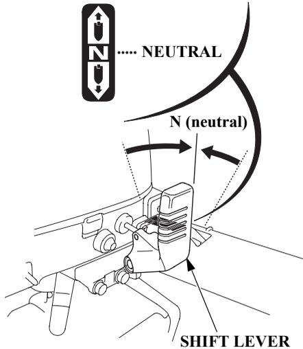
2. Move the shift lever to the N (neutral) position. The engine does not start unless the shift lever is set in the N (neutral) position.
