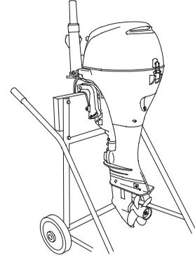
2. Transport the outboard motor with the tiller handle raised.
