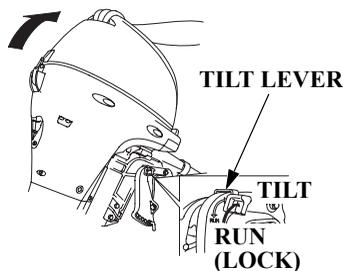
Use the tilt lever to temporarily raise the outboard motor when the boat is sailing in the shallows, or mooring or anchoring in the shallows. Raising the tilt lever unlocks the outboard motor and the outboard motor can be tilted. Lowering the tilt lever locks the outboard motor.
