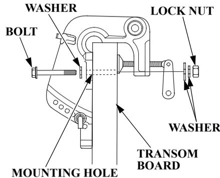
2. Apply the silicone sealant (Three Bond 1216 or equivalent) to the outboard motor mounting holes.
