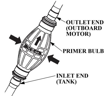
3. Hold the primer bulb so that the outlet end is higher than the inlet end. The arrow on the primer bulb points upward. Squeeze the primer bulb several times until it feels firm, indicating that fuel has reached the carburetor. Check for fuel leaks and repair any leaks before starting the engine.
