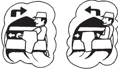
The boat swings its stern in the opposite direction in which it is to turn. To turn to the right, swing the steering handle to the left. To turn to the left, swing the steering handle to the right.
