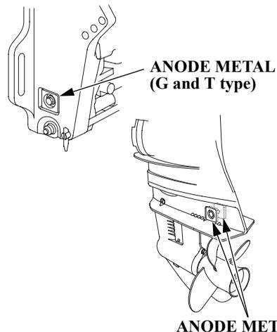
The anode metal is a sacrificed metal which protects the outboard motor from corrosion.
