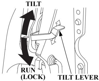
Use the tilt lever to temporarily raise the outboard motor when the boat is sailing in the shallows, or mooring or anchoring in the shallows. Raising the tilt lever unlocks the outboard motor and the outboard motor can be tilted. Lowering the tilt lever locks the outboard motor.
