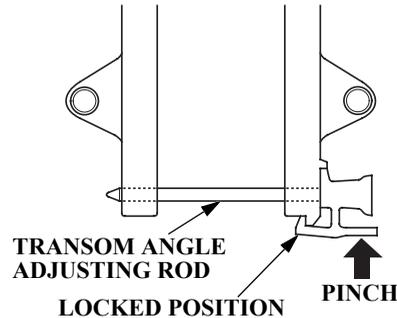
Pinch the adjusting rod end and pull out to remove.
