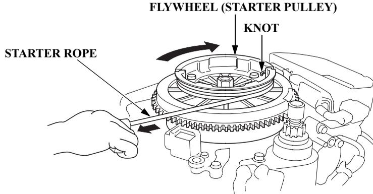
10. Set the knot at the end of the emergency starter rope in the notch in the flywheel, and while pulling the emergency starter rope clockwise around the flywheel.
