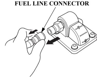
2. While pulling the fuel line connector cover, pull the fuel line connector to disconnect the fuel line connector from the fuel tank.
