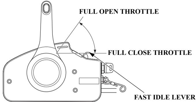
The fast idle lever is provided with the engine speed adjustment function. The lever does not move unless the remote control lever is in the “N” (neutral) position. Note also that the control lever does not move unless the fast idle lever is in the “full close” position.
