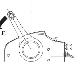
While pulling the neutral release lever, move the control lever 32° toward the FORWARD or REVERSE position to engage the clutch. Moving the control lever further opens the throttle and the engine speed increases.
