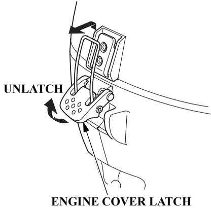
2. Unlatch the engine cover latch and remove the engine cover.
