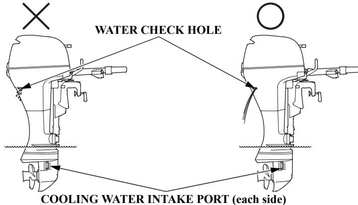
8. After starting, check whether the cooling water is flowing out of the cooling water check hole. Amount of water flowing out of the check hole might vary due to the thermostat operation, but this is normal.
