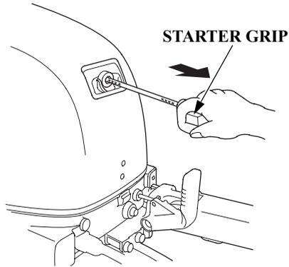
Pulling the starter grip operates the recoil starter to crank the engine for starting. Set the shift lever in the N (neutral) position before starting.
