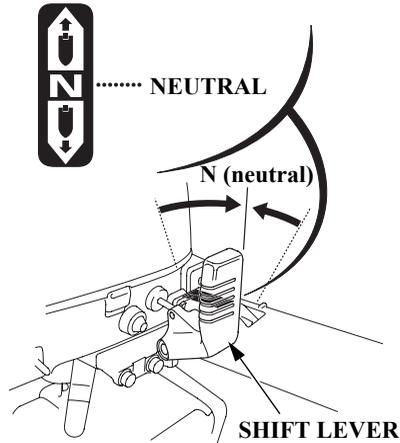
1. Move the shift lever to the N (neutral) position and stop the engine.
