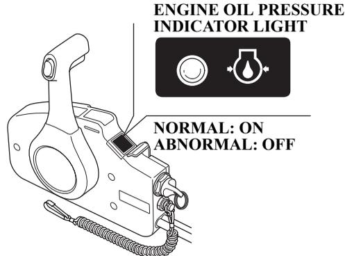
7. Check to see if the oil pressure indicator light turns ON.
