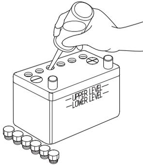
3. Fill the battery with distilled water to the upper level line. Never overfill the battery.
