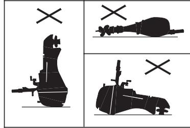
Rest the outboard motor on the case protector. (Tiller handle upside)
