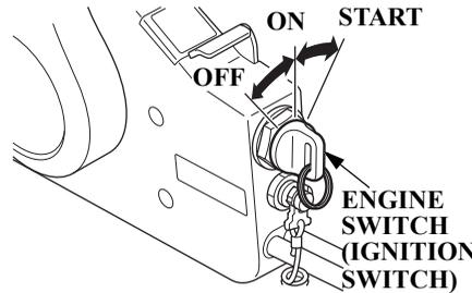
This remote control is equipped with an automotive type ignition switch.
