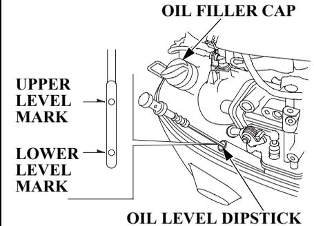
1. Position the outboard motor vertically, and remove the engine cover.
