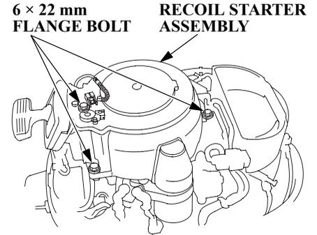
3. Remove the three 6 x 22 mm flange bolts and recoil starter assembly.
