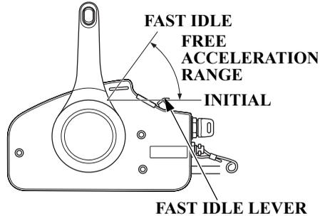
3. When the engine is cold or the ambient temperature is low, leave the fast idle lever in the initial position. (This will provide rich fuel mixture to the engine by the automatic choke.)
