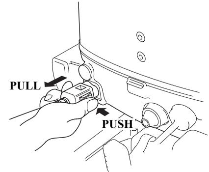
1. Disconnect the fuel line connector from the outboard motor.
