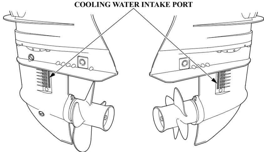
The engine cooling water is drawn into the engine through this port.
