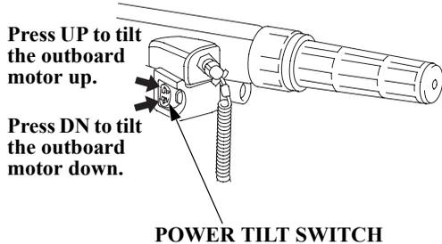
Excessive trim angle can result in cavitation and racing of the propeller, and tilting up the outboard motor excessively can cause damage to the impeller pump.
