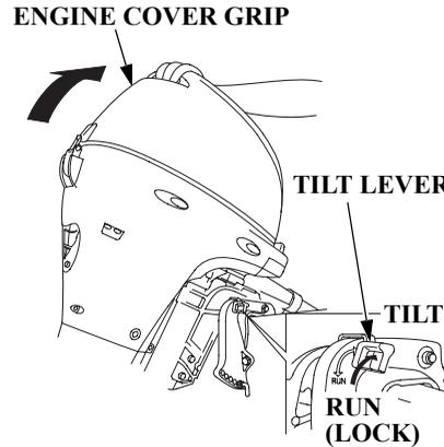
2. Move the tilt lever to the “TILT” position. Hold the engine cover grip and raise the outboard motor.
