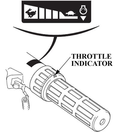
The curve on the grip label indicates the engine speed.
