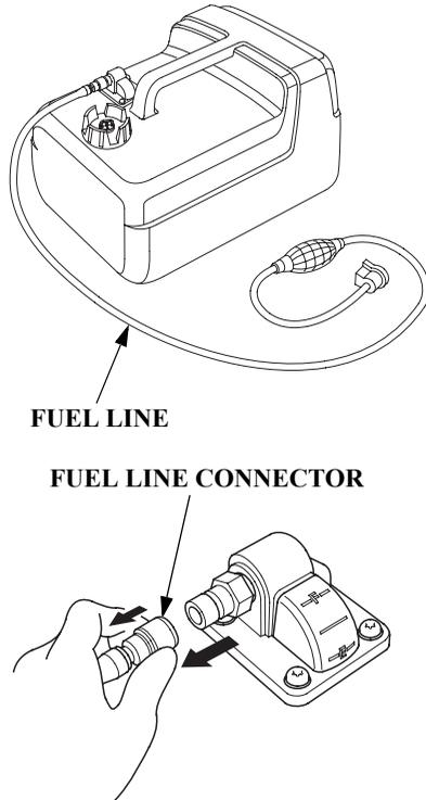
Clean the fuel tank and tank filter every year or after every 200 hours of outboard motor operation.
