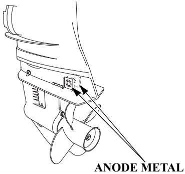
The anodes are a sacrificial material which helps to protect the outboard motor from corrosion.
