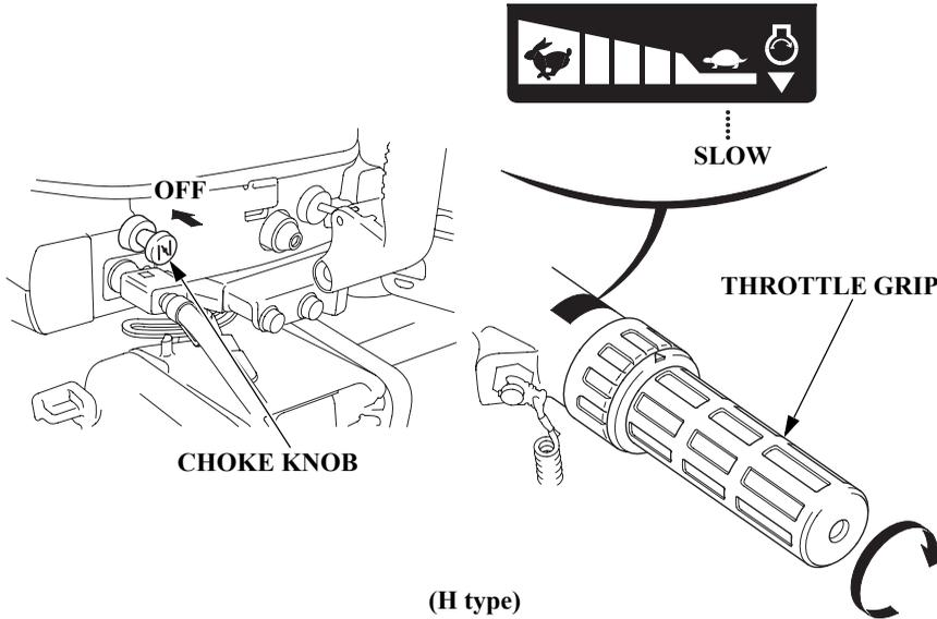
13. If you pulled out the choke knob to the ON position to start the engine, return it slowly to the OFF position (manual choke type), and turn the throttle grip in the SLOW direction to a position where the engine does not stall.
