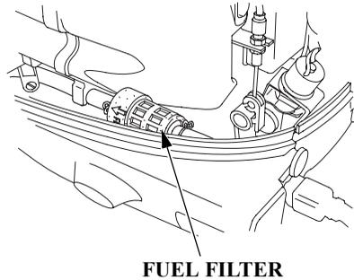
3. Check the fuel filter for water accumulation and clogging.
