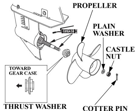
If the propeller is damaged by striking a rock, or other obstacle, replace the propeller as follows.
