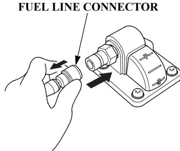
Inspect the fuel line, and the O-ring seals in the fuel line connectors. Replace the fuel line, or fuel line connectors if they are cracked, damaged or leak fuel. Be sure the fuel line is not kinked.
