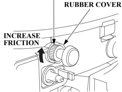
To adjust the friction, squeeze the rubber cover to grip the adjusting nut and turn it clockwise to increase the friction. Do not force the adjusting nut. If it is too hard to turn by hand, contact an authorized Honda Outboard Motor dealer for assistance.
