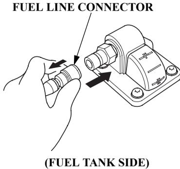
The fuel line connector is used to connect the fuel line between the separate fuel tank and the outboard motor.
