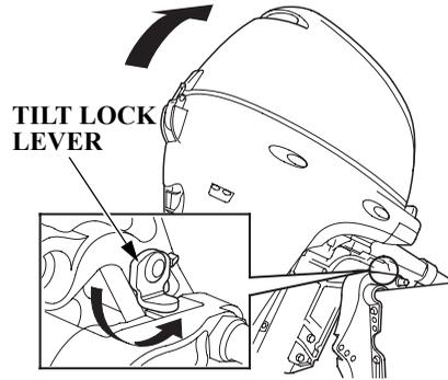
Tilt-up using the tilt lock lever.
