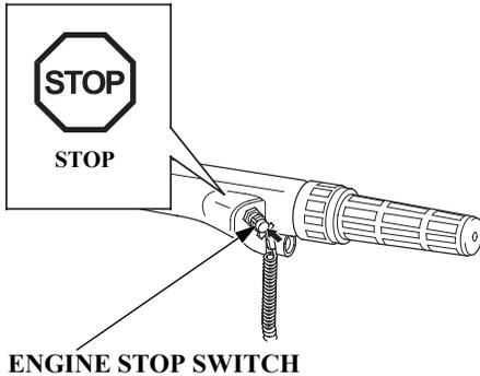
2. Press the engine stop switch until the engine stops.
