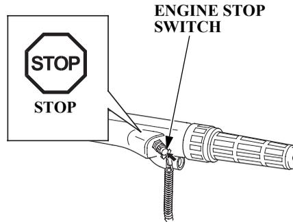
Press the engine stop switch to stop the engine.
