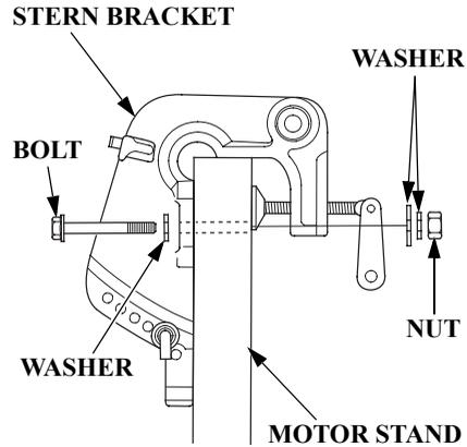
1. Attach the stern brackets to a motor stand and mount the outboard motor to the brackets.
