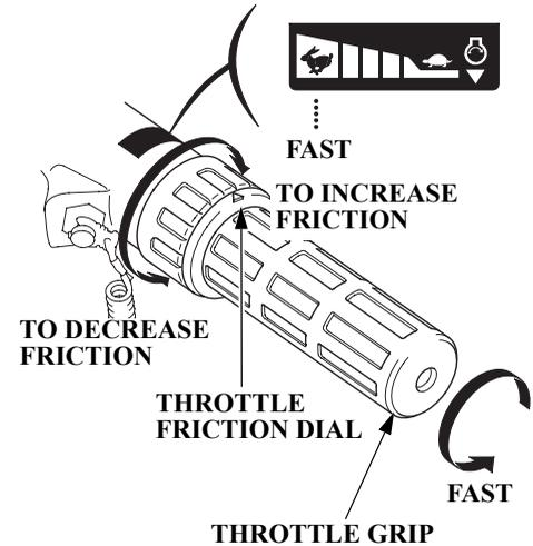
To hold the throttle at a steady setting, turn the throttle friction dial clockwise. To free the throttle grip for manual speed control, turn the friction dial counterclockwise.
