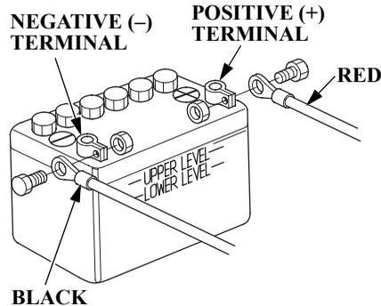
1. Disconnect the battery cable at the battery negative (-) terminal, then at the battery positive (+) terminal.
