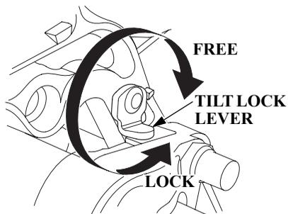
Use the tilt lock lever to raise the outboard motor and lock it in the position when the boat is moored or anchored for a long time. Tilt the outboard motor as far as it goes and move the lock lever in the locking direction.
