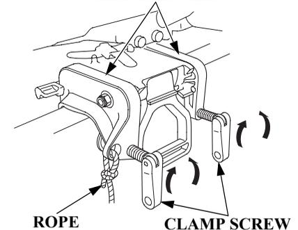
1. Attach the stern bracket to the transom and tighten the clamp screws. Push the carrying handle into the storage position.
