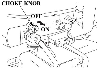
The choke knob opens and closes the choke valve in the carburetor.
