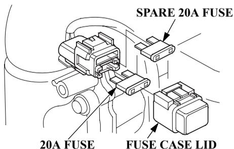
If the fuse blows, running the engine will not charge the battery. Before replacing the fuse, check the current ratings of the electrical accessories and ensure that there are no abnormalities.
