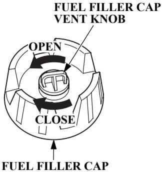
The vent knob shuts off the fuel tank from the open air.
