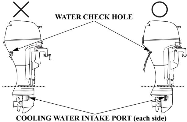
6. After starting, check whether the cooling water is flowing out of the cooling water check hole. Amount of water flowing out of the check hole might vary due to the thermostat operation, but this is normal.
