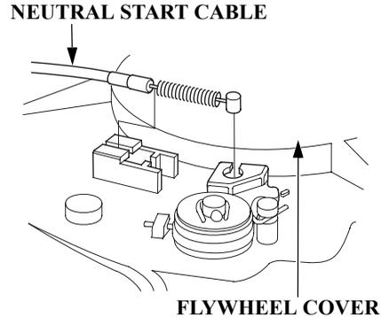
2. Move the shift lever to "F" (forward) position. Loosen the neutral start cable lock nut and disconnect the neutral start cable.
