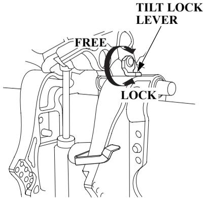
Tilt-up using the tilt lock lever.
