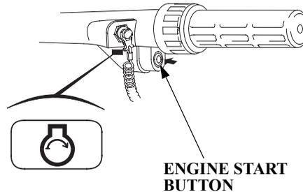
Use the engine start button to start the engine. Set the shift lever in the N (neutral) position before starting.
