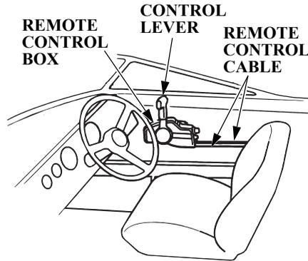
Install the remote control box in the position where is easy to operate the control lever and switches. Be sure that there are no obstacles on the route of the control cable.
