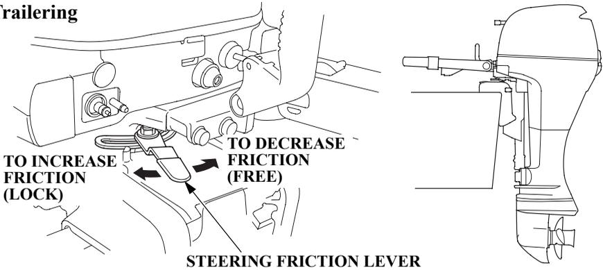
When trailering or transporting the boat with the outboard motor attached always disconnect the fuel line from the portable fuel tank and move the steering friction lever locked position.
