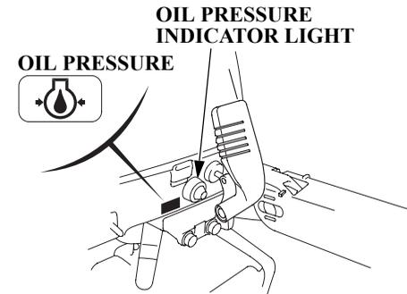
When the engine oil level is low or the engine lubrication system is faulty, the oil pressure indicator light turns off.
