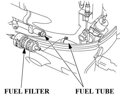
1. Remove the fuel filter, disconnect the right and left fuel lines, and replace with a new fuel filter.
