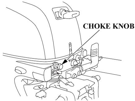
If the choke knob returns to the OFF position by itself, you can adjust the friction that holds the knob in the ON position.
