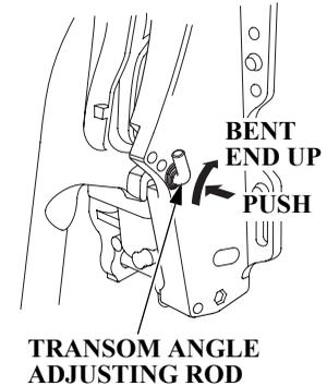
Push in the adjusting rod, twist upwards to the unlocked position and pull out to remove.
