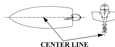
Install the outboard motor at the stern, at the center line of the boat.
