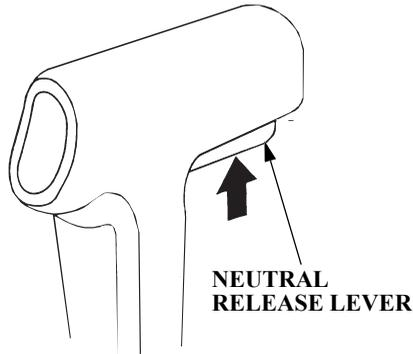
The neutral release lever is set on the remote control lever to prevent an accidental operation of the remote control lever.
