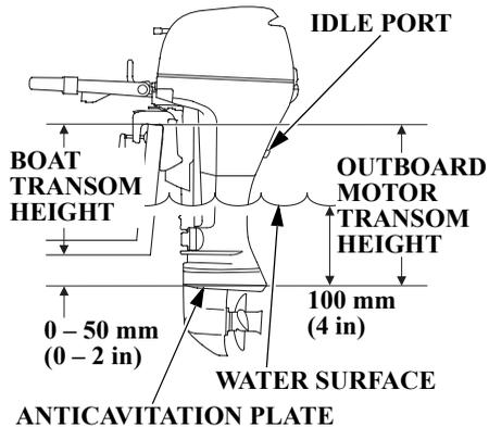
If the outboard motor is installed too low, the boat will squat and be hard to plane, and the engine will spray water that may enter the boat. It will tend to porpoise, and high-speed stability will be reduced.
