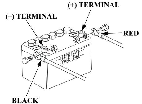
1. Disconnect the battery cable at the battery negative (-) terminal, then at the battery positive (+) terminal.
