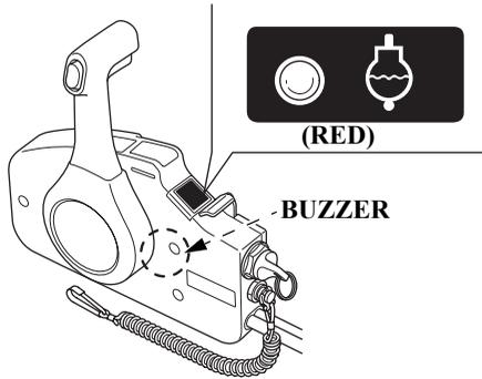
The overheat warning light turns on and the buzzer sounds when the engine cooling circuit is faulty. The engine speed slows down this time.
