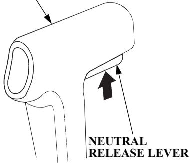
Shifting gear into forward, reverse, or neutral and the engine speed adjustment can be performed with the remote control lever.
