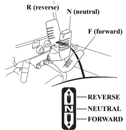
Use the shift lever to run the boat in forward or reverse gear, or to cut off the engine power from the propeller. There are three positions for the shift lever.
