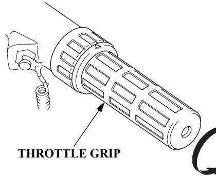
Turn the grip clockwise or counterclockwise to adjust the engine speed. Turning the grip in the direction shown by arrow increases the engine speed.
