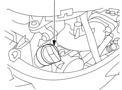
Drain the oil while the engine is still warm to assure rapid and complete draining.
