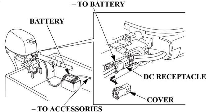
The DC receptacle provides a 12 volt, 6 amp. output for battery charging. The charging circuit is protected by a 20 amp. fuse that is accessible by removing the engine cover. A male plug for the DC receptacle is provided with the outboard motor; connect your battery charging wires to that plug. Be sure that the positive (Red) battery cable is connected to the (+) plug terminal.
