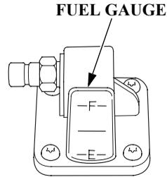
The fuel gauge indicates the fuel level in the tank.
