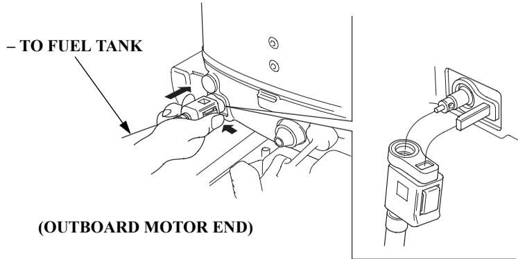
2. Connect the fuel line connector to the outboard motor. Install the outboard motor end fuel line connector with the clip toward the shift lever side. Be sure the fuel line connector is securely snapped in place. Always disconnect the fuel line when storing or transporting the outboard motor.
