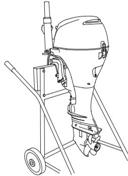
Transport and store the outboard motor either vertically or horizontally, as shown here. Store the outboard motor in a well-ventilated area free from direct sunlight and humidity.
