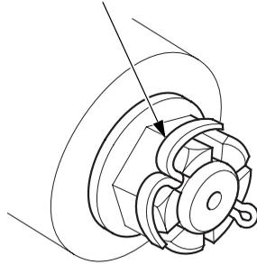
2. Install the new propeller in the reverse sequence to removal. Be sure to replace the coter pin with a new one.
