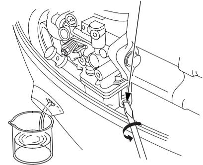
into a suitable container, then retighten the carburetor drain screw (see page 133).
