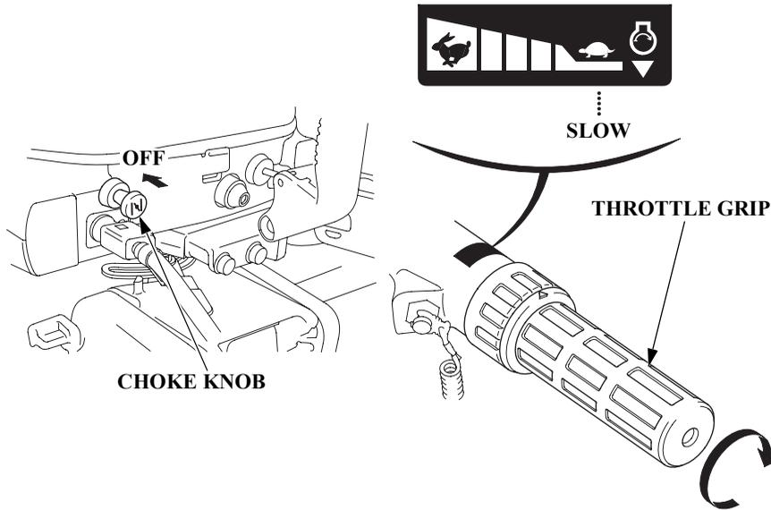
7. If you pulled out the choke knob to the ON position to start the engine, return it slowly to the OFF position (manual choke type), and turn the throttle grip in the SLOW direction to a position where the engine does not stall.
