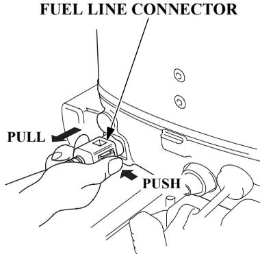
1. While pressing the fuel line connector clip, pull the fuel line connector and disconnect it from the outboard motor side joint.
