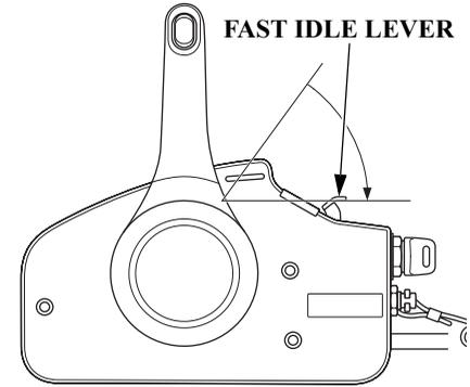
12. If the fast idle lever is raised, return the fast idle lever slowly to the position where the engine does not stall and hold the lever in the position.
