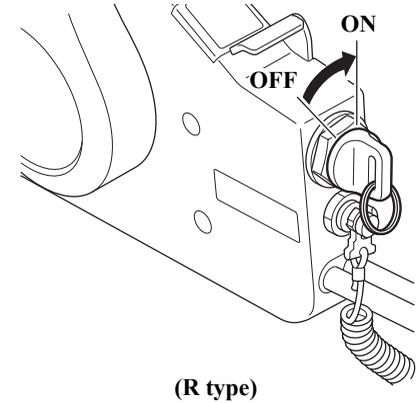
6. If your outboard motor is the remote control type, turn the engine stop switch to the "ON" position.
