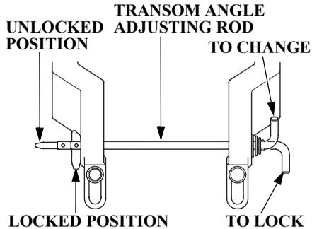
Inserting the adjusting rod in the proper hole, twist it down to lock. After locking, pull the adjusting rod and be sure it is not withdrawn.
