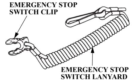
The emergency stop switch lanyard is provided to stop the engine immediately when the operator falls overboard or away from the outboard motor.
