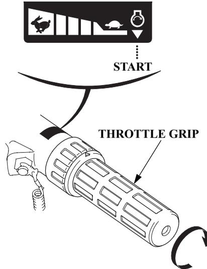
3. Align the “
