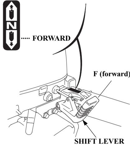
1. With the shift lever in the FORWARD position, turn the throttle grip in the FAST direction to increase the speed.
