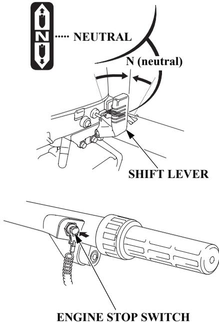
1. Move the shift lever or the control lever to the N (neutral) position and stop the engine.
