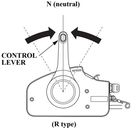
4. Set the shift lever/control lever in the N (neutral) position.
