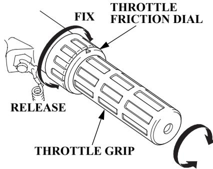
Use the engine throttle fixing dial to cruise at a certain constant speed. Turning the fixing dial clockwise fixes the throttle grip in place, and it is released by turning the fixing dial counterclockwise.
