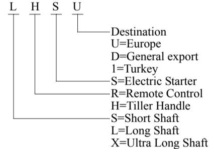
This Owner's Manual is using the following type names when it describes the operations special to a type.
