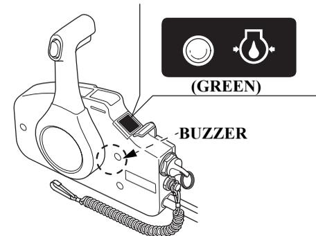
The oil pressure indicator light turns off and the buzzer sounds when the oil level is low and/or the engine lubrication system is faulty.
