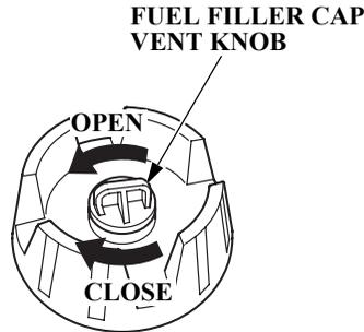
4. Turn the vent knob to OPEN side, squeeze and release the priming bulb to feed the fuel, and check for leaks.
