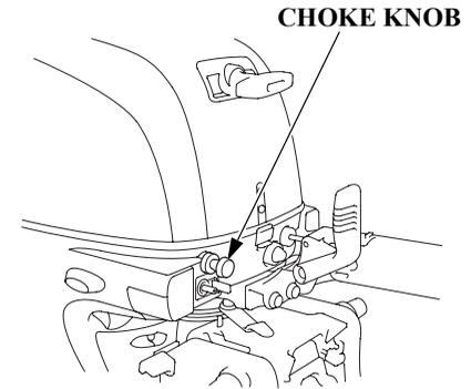
The maintenance procedure differs depending on which enrichment system you have. You can tell which system you have according to whether there is a choke knob.
