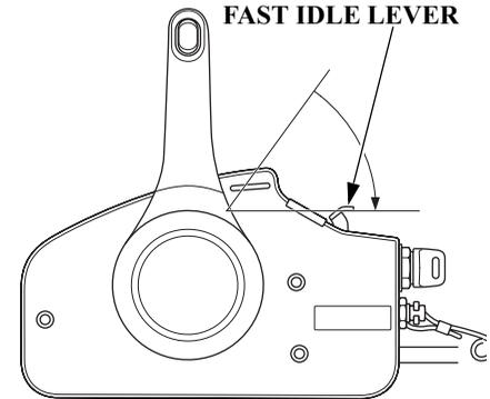
5. If the fast idle lever is raised, return the fast idle lever slowly to the position where the engine does not stall and hold the lever in the position.
