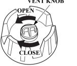
1. (When using the internal fuel tank) Open the fuel filler cap vent knob 2 to 3 turns counterclockwise.
