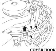
3. Release the throttle cables from the cover hook.
