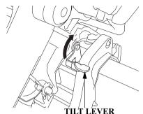
Use the tilt lever to temporarily raise the outboard motor when the boat is running in the shallows, or mooring or anchoring in the shallows. Raising the tilt lever unlocks the outboard motor and the outboard motor can be tilted. Lowering the tilt lever locks the outboard motor.
