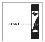
4. Align the "♂" mark on the throttle grip with the projected end of the "▶" mark on the handle.
