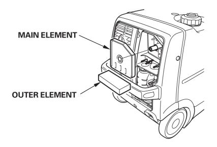
3. Wash the elements in a solution of household detergent and warm water and rinse thoroughly, or wash in nonflammable or high flash point solvent. Allow the elements to dry thoroughly. If the elements are damaged, replace them.
