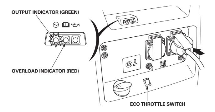
If you wish to use the Eco Throttle system, turn the Eco Throttle switch to the ECO position (see page 15).
