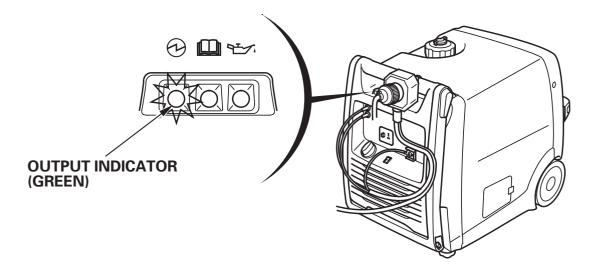
5. Confirm that the appliance to be used is switched off, and plug in the appliance.
