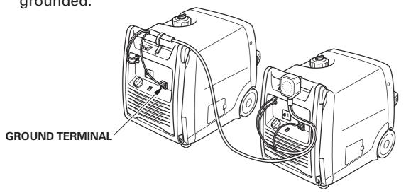
4. Start the engines and make sure the Output indicators (green) come on.
