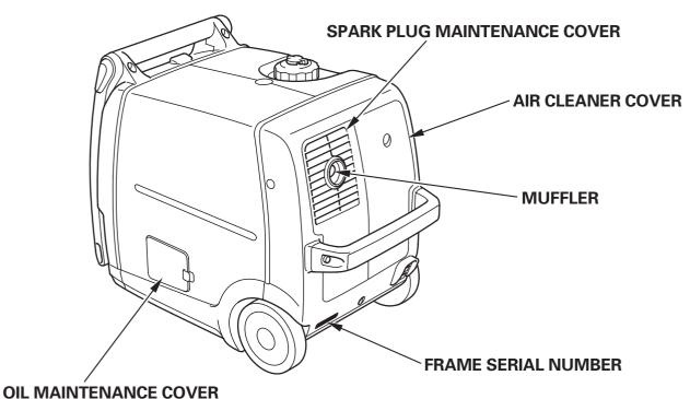
Record the frame serial number in the space below. You will need this serial number when ordering parts.
