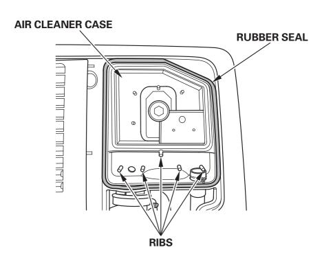
7. Reinstall the air cleaner cover and tighten the air cleaner cover screw securely.
