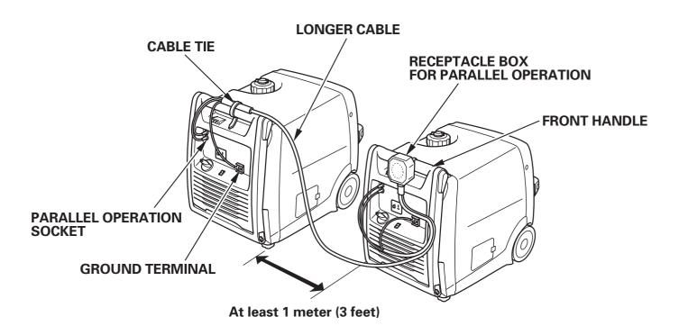
3. Be sure to ground the generator when the connected equipment is grounded.
