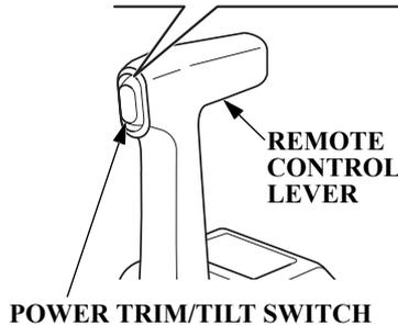
Consult an authorized Honda Outboard Motor dealer for the method to adjust the tilt limit switch. Press either UP or DN (down) of the power trim/tilt switch and tilt the outboard motor to the best position in compliance with the cruising conditions.
