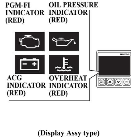
If the engine overheats, the engine will stop in 20 seconds after the engine protection system will limit engine speed. Each warning system of PGM-FI, ACG, oil pressure, overheat, and water separator is activated as described in the following table.
