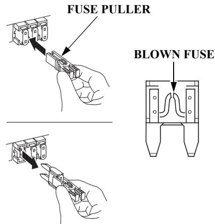
5. Pull the old fuse out of the clip with the fuse puller supplied in the fuse box.
