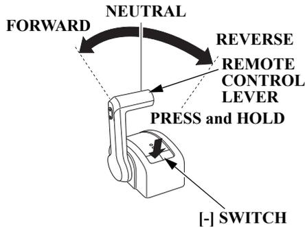
Use the [-] switch and the remote control lever to adjust the engine speed without gearshift when warming up the engine.
