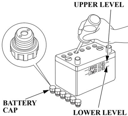
3. Fill the battery with distilled water to the upper level line. Never overfill the battery.
