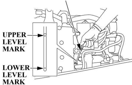
4. Refill to the upper level mark on the oil level dipstick with the recommended oil.
