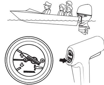
With the outboard motor trimmed high the trim meter will read as shown. To lower the bow decrease the outboard motor trim angle by pressing the DN (down) portion of the power trim/tilt switch.
