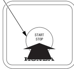
2. Push the start/stop switch to stop the engine.
