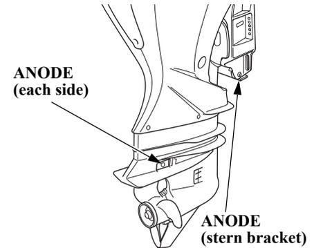
The anode is a sacrificial material which helps to protect the outboard motor from corrosion.
