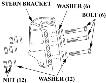
1. Apply the silicone sealant (Three Bond 1216 or equivalent) to the outboard motor mounting holes.
