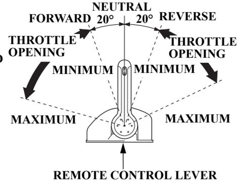
Shifting gear into forward, reverse, or neutral and the engine speed adjustment can be performed with the remote control lever.
