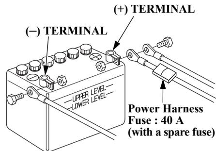
1. Disconnect the battery cable at the battery negative (-) terminal, then at the battery positive (+) terminal.
