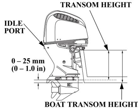
Make sure that the boat transom height is correct for the outboard motor. Incorrect installation height will reduce performance. The outboard motor should be installed so that the anticavitation plate is 0 - 25 mm (0 - 1.0 in) upper the bottom of the boat. The correct dimensions differ according to the type of the boats and the figuration of the bottom of the boats. Follow the manufacture's recommended installation height.
