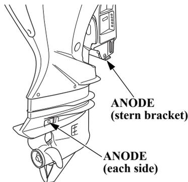
The anode is a sacrificial material which helps to protect the outboard motor from corrosion.
