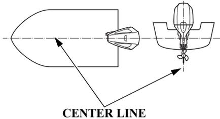
Install the outboard motor at the stern, at the center line of the boat.
