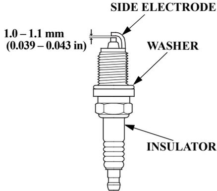
7. Measure the plug gaps with a feeler gauge. Correct the gap, if necessary, by carefully bending the side electrode.
