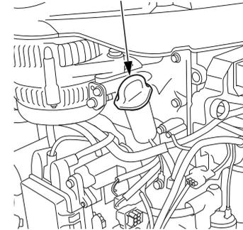
When the engine oil is contaminated or discolored, replace with the fresh engine oil (see page 119 for replacement interval and procedure).
