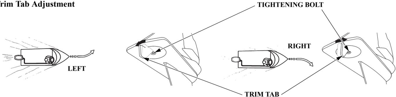
The trim tab is provided to adjust for “torque steer” which is a reaction of the propeller rotation or propeller torque. If during a high speed turn an unequal amount of effort is required to turn the boat right or left, adjust the trim tab so that an equal amount of effort is required.
