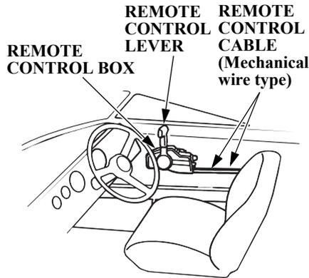
Install the remote control box in the position where is easy to operate the remote control lever and switches.
