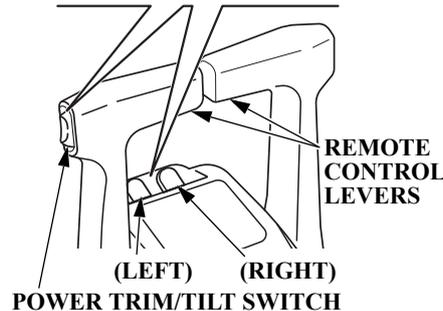
The power trim/tilt system operates when the switch is pressed, and it stops when the switch is released. To trim up slightly, press on UP momentarily but securely. To trim down slightly, press on DN (down) in the same manner.
