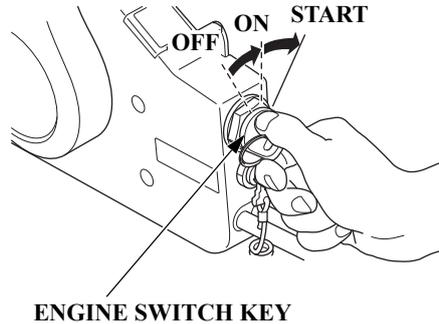
3. Turn the engine switch key to the START position and hold it there until the engine starts.
