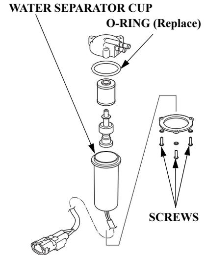
5. Remove the three screws holding the fuel filter with water separator, delete the water or deposit from the inside of the cup.
