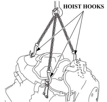
2. Set the hoist hooks against the lifting eyes and hang the outboard motor to remove it from the boat.
