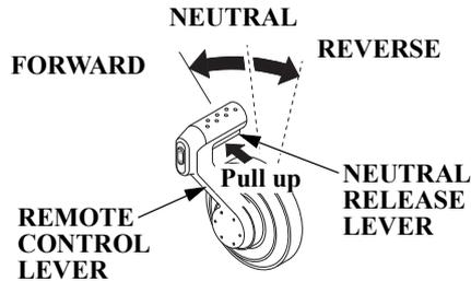
Use the [-] switch and the remote control lever to adjust the engine speed without gearshift when warming up the engine. Keeping the [-] switch pressed when the remote control lever is in the NEUTRAL position, turn the lever forward. Keep turning the lever forward. The throttle opens and the engine speed increases after the lever passed the shift point.
