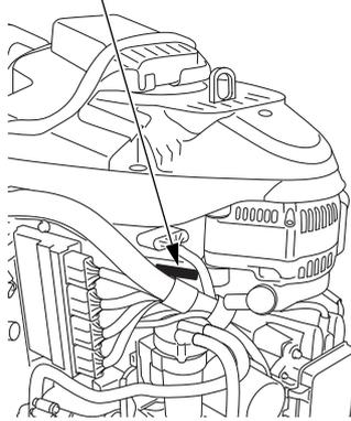
The engine serial number is stamped on the upper right side of the engine.
