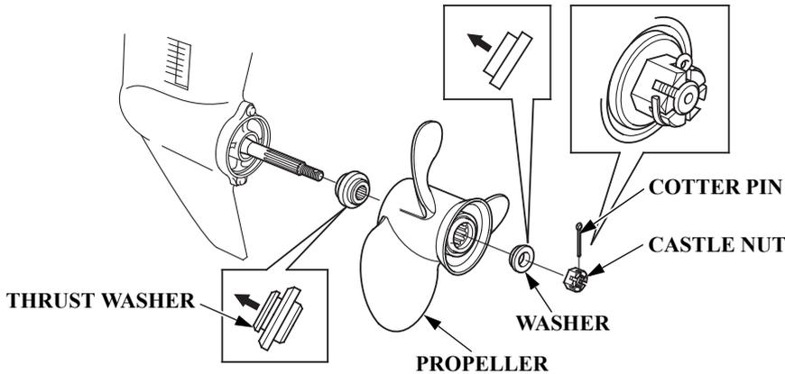
When replacing the propeller, put a suitable chip of wood between the propeller and the anticavitation plate to prevent the propeller from rotating.
