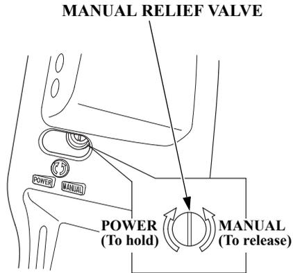
If the power trim/tilt switch will not tilt the outboard motor, the outboard motor can be manually tilted up or down by opening the manual relief valve. To tilt the outboard motor manually, turn the manual relief valve under the left stern bracket no more than 1 or 2 turns counterclockwise using a screwdriver.
