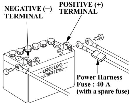
3. Connect the battery positive (+) cable to the battery positive (+) terminal, then the battery negative (-) cable to the battery negative (-) terminal. Tighten the bolts and nuts securely. Coat the battery terminals with grease.
