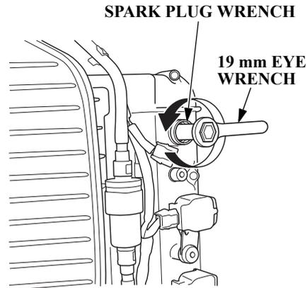
5. Use the spark plug wrench and 19 mm eye wrench to remove the spark plugs.
