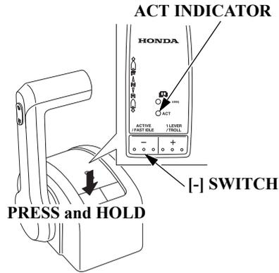
For multiple station type, use the [-] switch to change the operating station.
