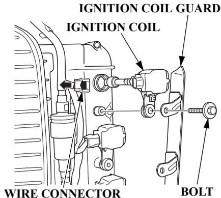
3. Disconnect the wire connector from the ignition coil by pushing on the lock tab and pulling on the connector. Pull on the plastic connector, not the wires.
