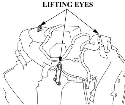
When transporting the outboard motor on a vehicle, perform the following.
