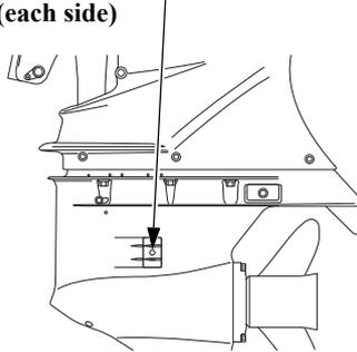
The engine cooling water is drawn into the engine through this port.
