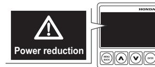
This outboard motor is equipped with the power reduction system which activates when the outboard motor has a serious problem.
