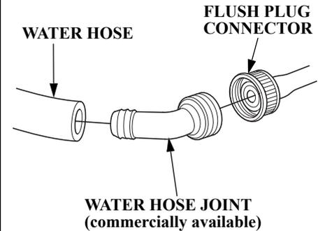
6. Connect a fresh water hose to the water hose joint.
