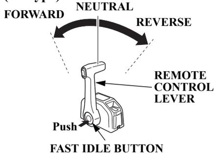
Use the fast idle button and the remote control lever to adjust the engine speed without gearshift when warming up the engine. Pushing the fast idle button, turn the remote control lever forward. Keep turning the lever forward. The throttle opens and the engine speed increases after the lever passed the shift point. Note that the gearshift mechanism does not function when the fast idle button is pushed once and then released after the remote control lever is moved.
