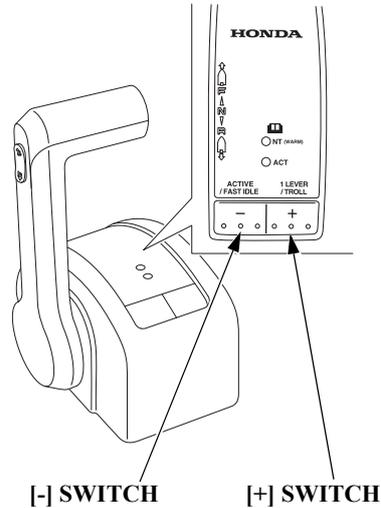
Function switches are used for operations in the fast idle mode, trolling mode, one-lever mode and station select mode.
