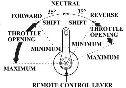
Shifting gear into forward, reverse, or neutral and the engine speed adjustment can be performed with the remote control lever.
