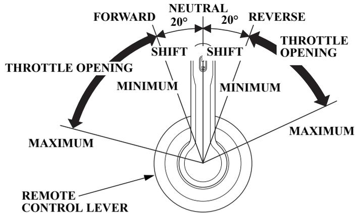
Shifting gear into forward, reverse, or neutral and the engine speed adjustment can be performed with the remote control lever.
