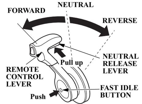
Pushing the fast idle button, turn the remote control lever forward. Keep turning the lever forward. The throttle opens and the engine speed increases after the lever passed the shift point. Note that the gearshift mechanism does not function when the fast idle button is pushed once and then released after the remote control lever is moved.
