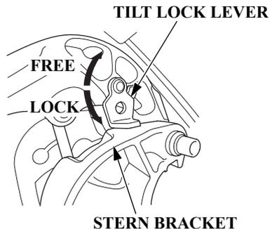
1. Raise the outboard motor as full as it goes using the power trim/tilt switch.
