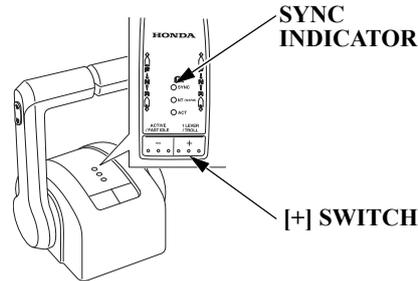
Shifting gear and the engine speed adjustment of the all outboard motors can be performed with one remote control lever when in one-lever mode.
