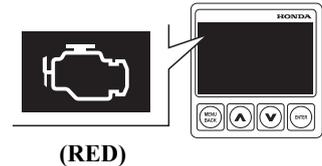
The PGM-FI indicator turns on and the buzzer sounds when the engine control system is faulty.
