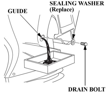
2. Place a suitable container under the guide.
