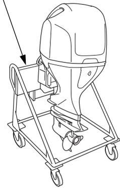
3. Secure the outboard motor on an outboard motor stand with the mounting bolts and nuts.
