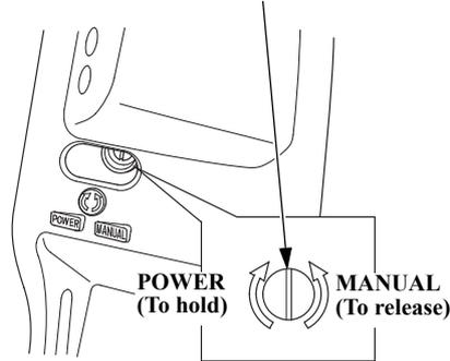
When power trim/tilt system does not operate because of dead battery or faulty power trim/tilt motor, the outboard motor can be manually tilted up or down by operating the manual relief valve.
