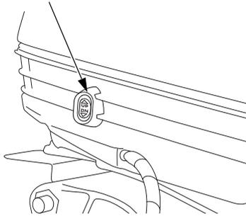
When you are away from the power trim/tilt switch on the control lever side, you can operate the power trim/tilt switch on the outboard motor side. The switch operation is the same as that of the switch on the control lever side.
