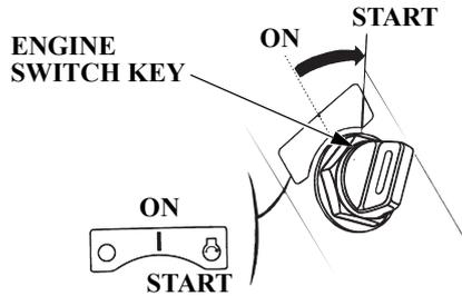
3. Turn the engine switch key to the START position and hold it there until the engine starts.
