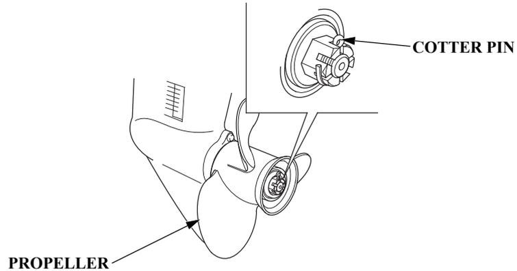
Engine speed varies according to the propeller size and the boat condition. Use of the outboard motor outside the full throttle speed range will adversely affect the engine and cause a serious problem. Use of the correct propeller assures powerful acceleration, top speed, excellency in terms of economy and cruising comfort, and it assures longer engine life as well.
