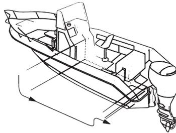
Measure the distance from the control box to the outboard motor along the cable routing.
