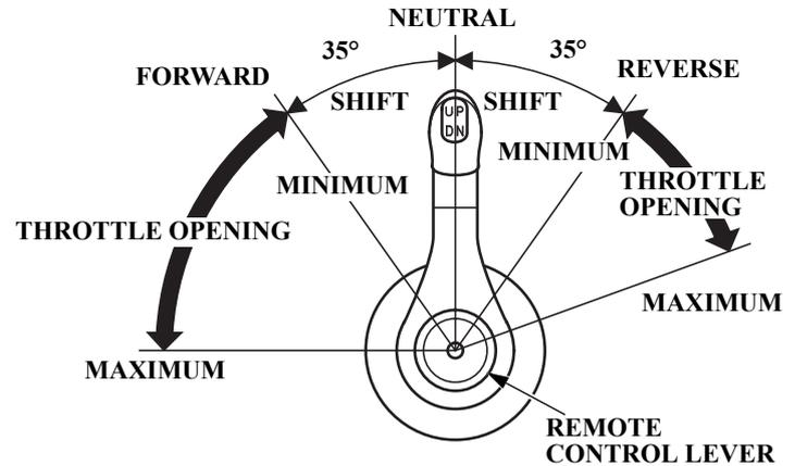
Shifting gear into forward, reverse, or neutral and the engine speed adjustment can be performed with the remote control lever.
