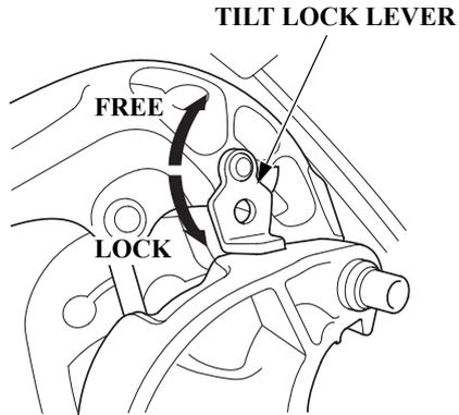
Use the tilt lock lever to raise the outboard motor and lock it in the position when the boat is moored or anchored for a long time.
