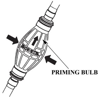
Hold the priming bulb so that the outlet end is higher than the inlet (so that the arrow on the priming bulb points up), and squeeze it until it feels firm, indicating that fuel has reached the outboard motor. Check for leaks.
