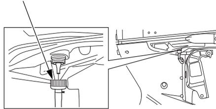
4. Remove the flush plug connector from the outboard motor.
