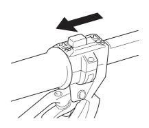
2. Turn the choke lever to the close position, if necessary.
