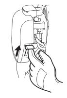
3. Press the priming pump several times until fuel stays in a priming pump.
