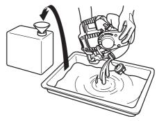
2. Press the priming pump several times and drain the fuel from the fuel tank again.
