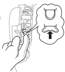
3. Remove the oil filler cap and drain the oil. 拆下機油加注口蓋並排掉機油。
