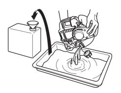
3. Pull out the fuel filter and clean it gently. 拉出燃油濾清器並小心地清潔。
