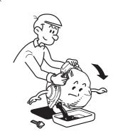
4. Fill the oil to the edge of the oil filler neck. 請添加機油至機油加注口邊緣。
