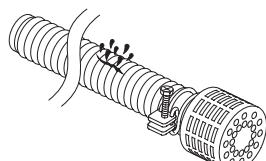
Is the hose band installed securely?
