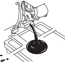
4. Tighten the oil drain plug and fill the oil to the oil filler neck.
