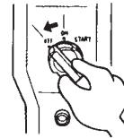
3. Turn the fuel valve to the “OFF” position.
