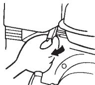
3. Turn the choke lever to the close position.
