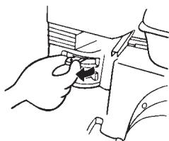
4. Turn the engine switch to the "ON" position.
