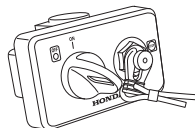
NORMAL KEY WITH START/STOP SWITCH TYPE
