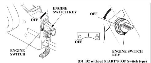
2. Turn the engine switch key to the OFF position to stop the engine.
