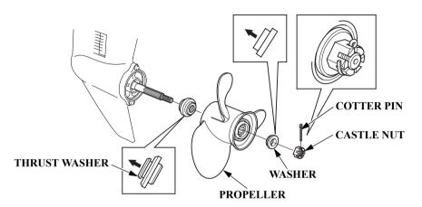
When replacing the propeller, put a suitable chip of wood between the propeller and the anticavitation plate to prevent the propeller from rotating.
