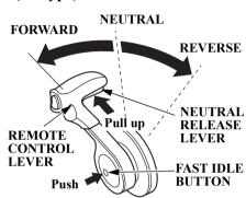
Pushing the fast idle button, turn the remote control lever forward. Keep turning the lever forward. The throttle opens and the engine speed increases after the lever passed the shift point. Note that the gearshift mechanism does not function when the fast idle button is pushed once and then released after the remote control lever is moved.
