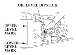
4. Refill to the upper level mark on the oil level dipstick with the recommended oil.
