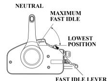
The fast idle lever will not move unless the remote control lever is in the NEUTRAL position. Conversely, the remote control lever will not move unless the fast idle lever is in the lowest position.
