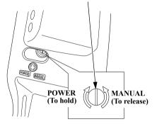
When power trim/tilt system does not operate because of dead battery or faulty power trim/tilt motor, the outboard motor can be manually tilted up or down by operating the manual relief valve.
