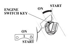
3. Turn the engine switch key to the START position and hold it there until the engine starts.
