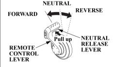
Use the [-] switch and the remote control lever to adjust the engine speed without gearshift when warming up the engine.
