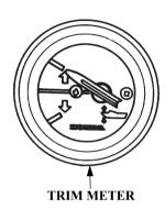
The trim meter has a range of  $-4^{\circ}$  to  $16^{\circ}$  and indicates the trim angle of the outboard motor. Refer to the trim meter when using the power trim/tilt switch to achieve proper boat performance.
