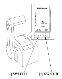
Function switches are used for operations in the fast idle mode, trolling mode, one-lever mode and station select mode.
