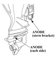
The anode is a sacrificial material which helps to protect the outboard motor from corrosion.
