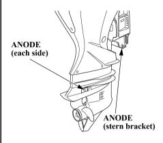
The anode is a sacrificial material which helps to protect the outboard motor from corrosion.
