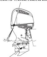
**COOLING WATER INTAKE PORT** (each side)
