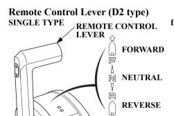
Shifting gear into forward, reverse, or neutral and the engine speed adjustment can be performed with the remote control lever.
