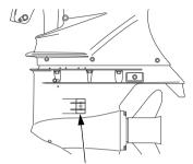
**COOLING WATER INTAKE PORT** (each side)
