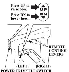
The power trim/tilt system operates when the switch is pressed, and it stops when the switch is released. To trim up slightly, press on UP momentarily but securely. To trim down slightly, press on DN (down) in the same manner.
