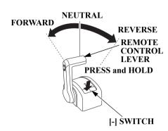
Use the [-] switch and the remote control lever to adjust the engine speed without gearshift when warming up the engine.
