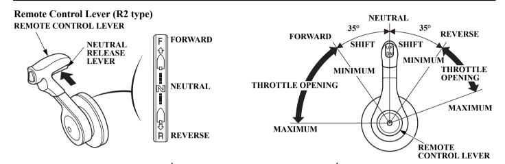
Shifting gear into forward, reverse, or neutral and the engine speed adjustment can be performed with the remote control lever.
