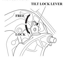
Use the tilt lock lever to raise the outboard motor and lock it in the position when the boat is moored or anchored for a long time.
