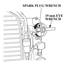
5. Use the spark plug wrench and 19 mm eye wrench to remove the spark plugs.
