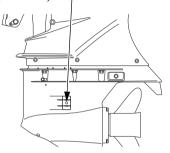
The engine cooling water is drawn into the engine through this port.
