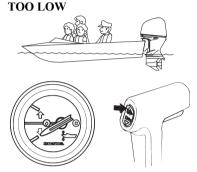
With the outboard motor trimmed low the trim meter will read as shown. To raise the bow increase the outboard motor trim angle by pressing the UP portion of the power trim/tilt switch.
