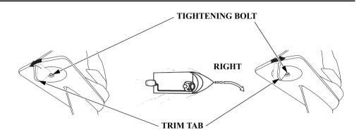
The trim tab is provided to adjust for "torque steer" which is a reaction of the propeller rotation or propeller torque. If during a high speed turn an unequal amount of effort is required to turn the boat right or left, adjust the trim tab so that an equal amount of effort is required.
