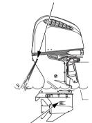
COOLING WATER INTAKE PORT (each side)
