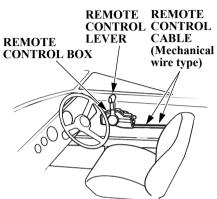
Install the remote control box in the position where is easy to operate the remote control lever and switches. Mechanical wire type:
