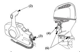
The anode (sacrificed metal) helps to protect the outboard motor from corrosion damage; it must be exposed directly to the water whenever the outboard motor is in use. Replace the anodes when they have been reduced to about two-thirds of their original size, or if they are crumbling.
