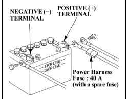
3. Connect the battery positive (+) cable to the battery positive (+) terminal, then the battery negative (-) cable to the battery negative (-) terminal. Tighten the bolts and nuts securely. Coat the battery terminals with grease.
