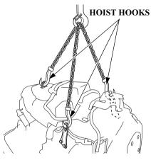
2. Set the hoist hooks against the lifting eyes and hang the outboard motor to remove it from the boat.
