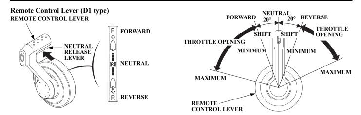
Shifting gear into forward, reverse, or neutral and the engine speed adjustment can be performed with the remote control lever.
