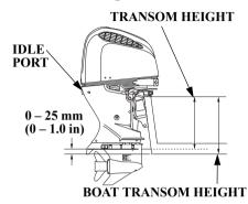
Make sure that the boat transom height is correct for the outboard motor. Incorrect installation height will reduce performance. The outboard motor should be installed so that the anticavitation plate is 0-25 mm (0-1.0 in) upper the bottom of the boat. The correct dimensions differ according to the type of the boats and the figuration of the bottom of the boats. Follow the manufacture's recommended installation height.
