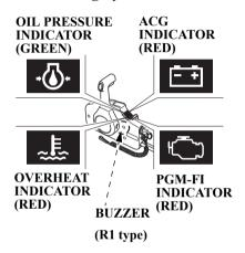
If the engine oil pressure drops and/ or the engine overheats, either or both warning systems could be activated. When activated the engine speed will decrease gradually and the green oil pressure indicator will turn OFF and the red overheat indicator will turn ON. A continuous buzzer will sound
