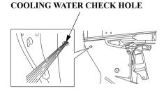
The cooling water is checked here to see whether it is circulating inside the engine properly.
