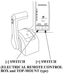
[-] Switch: Reduce engine speed [+] Switch: Increase engine speed
