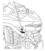
The engine serial number is stamped on the upper right side of the engine.
