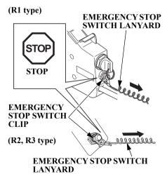
Pull the curl cord of the emergency stop switch and remove the lock plate from the switch; this will stop the engine.
