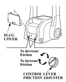
Check whether the remote control lever moves smoothly. Friction of the lever can be adjusted by turning the control lever friction
