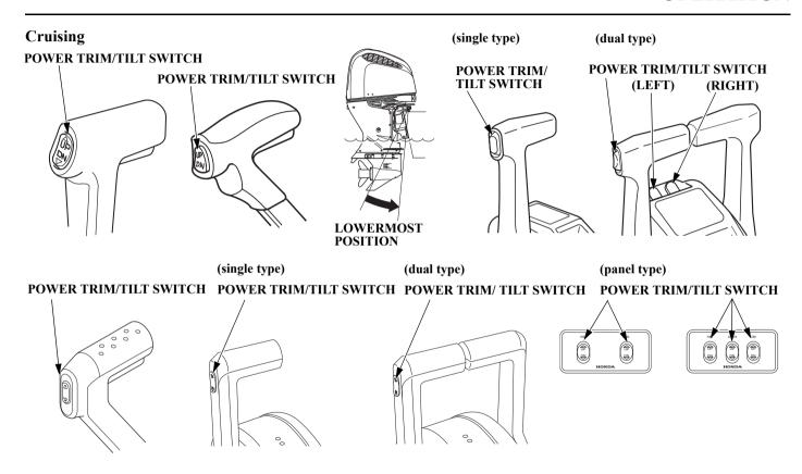
1. Press on the DN (down) of the power trim/tilt switch and trim the outboard motor at the lowermost position.
