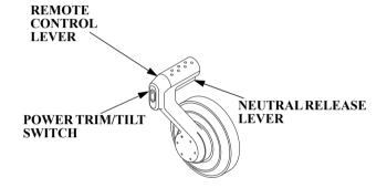
**TOP-MOUNT TYPE (D2 type)** (SINGLE OUTBOARD MOTOR TYPE)
