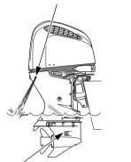
**COOLING WATER INTAKE PORT** (each side)
