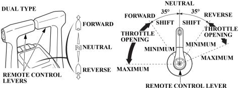
Shifting gear into forward, reverse, or neutral and the engine speed adjustment can be performed with the remote control lever.
