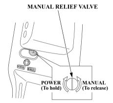
After tilting the outboard motor, turn the manual relief valve clockwise securely.
