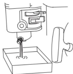
3. Remove the drain plug and drain the oil.
