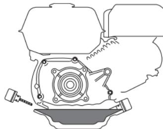
3. Install the oil drain plug and sealing washer. Tighten the oil drain plug and fill the oil to the edge of the oil filler neck.
