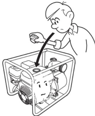
2. If the fuel level is low. Refill the tank.
