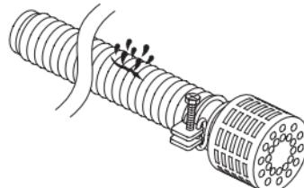
Is the hose band installed securely?
