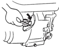
5. Pull the starter grip lightly until resistance is felt, then pull briskly.
