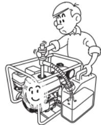
**2. Loosen the drain bolt by turning it 1 to 2 turns counter clockwise and drain the fuel from the carburetor.**
