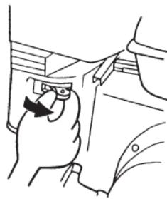
7. Set the throttle lever at the desired position.
