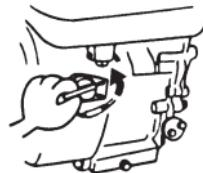
3. Turn the fuel valve to the “OFF” position.
