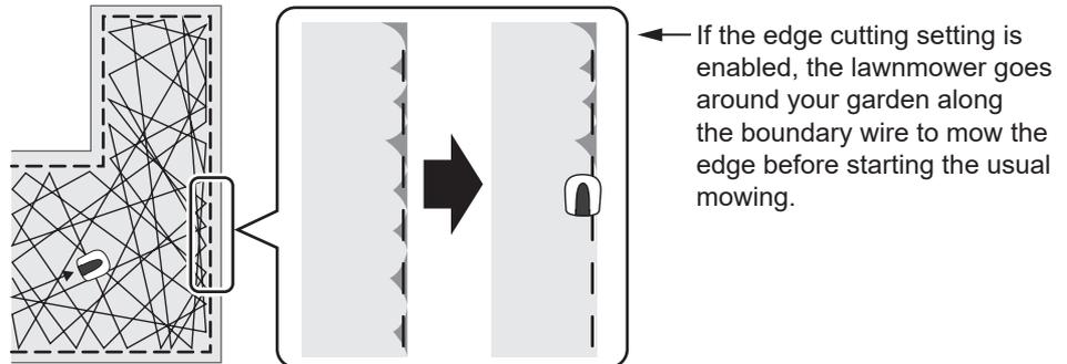
If you set this function on, the lawnmower mows along the boundary wire when the work timer starts for the first time on selected day(s). You can also configure the day(s) of the week on which you want the lawnmower to mow along the boundary wire (2 days per week maximum).
