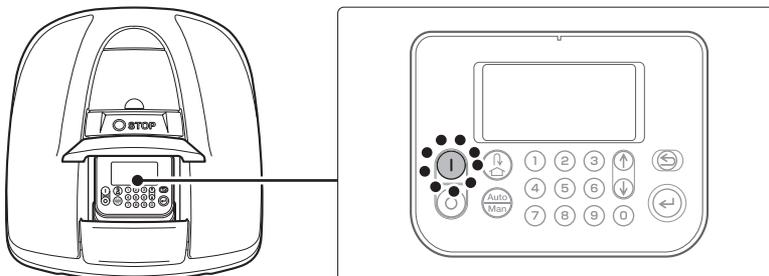
The power turns on, and the initial setup screen on the control panel is displayed.
