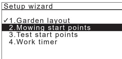
**2-2** Select [Yes] or [No] to the question on the addition of the start points and press the button. If you select [Yes], go to step 2-3. If you select [No], no start point is added and the setup wizard top screen is displayed.
