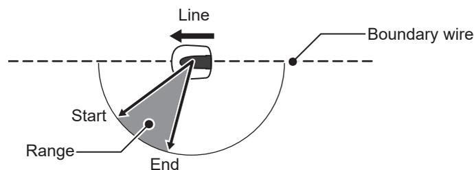
**TIPS** Use the exit angle to let the lawnmower reach the mowing areas directly instead of using long wire exit locations.
