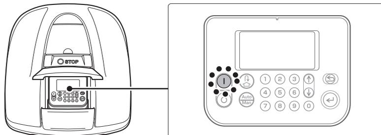
The power turns on, and the startup screen on the control panel is displayed.
