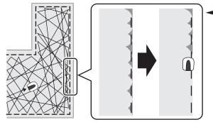
If the edge cutting setting is enabled, the lawnmower goes around your garden along the boundary wire to mow the edge before starting the usual mowing.
