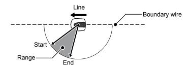
Use the exit angle to let the lawnmower reach the mowing areas directly instead of using long wire exit locations.
