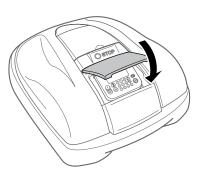
When the lawnmower is docked at the docking station, press the manual STOP button. The control panel cover pops up.
