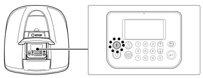
The power turns on, and the initial setup screen on the control panel is displayed.
