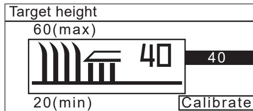
**2** Set the “Start cutting height” with the ▲▼ buttons or number buttons and press the ⏪ button.
