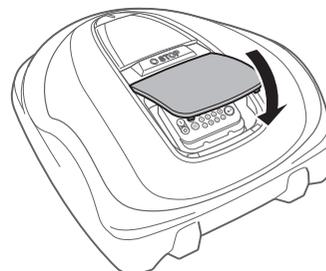
**4-5** Press the manual STOP button. The control panel cover pops up. The message “Do you want to modify the start point?” appears on the display.
