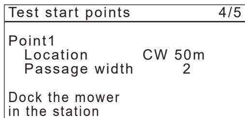
**4-4** Close the control panel cover. The lawnmower starts towards the selected start point. When the test is correctly finished, the lawnmower rolls slowly from the minimum to the maximum exit angle, and a beep sound is emitted from the lawnmower.
