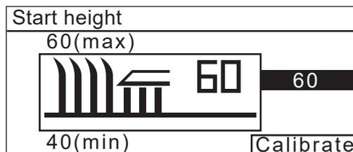
4 When you select [Calibrate] and press the
