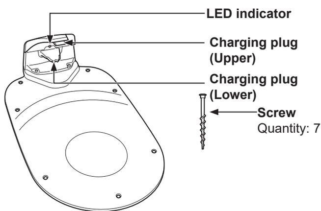
The lawnmower recharges at the docking station, and returns to the docking station when mowing is finished or the battery's charge becomes low. You can check the status of the boundary wire with the LED indicator (☞ page 67).
