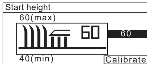
**3** When you select [Calibrate] and press the ⏪ button, the blade disc moves to the set cutting height. You can check the cutting height.
