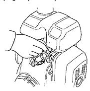
5. After the spark plug is seated, tighten with a spark plug wrench to compress the washer.
