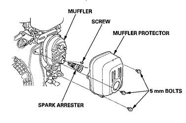
Use a brush to remove carbon deposits from the spark arrester screen.
