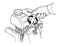
2. Visually inspect the spark plug. Discard the spark plug if there is apparent wear, or if the insulator is cracked or chipped. Clean the spark plug with a wire brush if it is to be reused.
