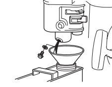
3. Remove the drain plug and drain the oil.
