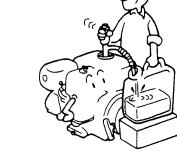
2. Drain the fuel from the carburetor.
