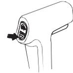
With the outboard motor trimmed high the trim meter will read as shown. To lower the bow decrease the outboard motor trim angle by pressing the DN (down) portion of the power trim/tilt switch.
