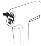
With the outboard motor trimmed low the trim meter will read as shown. To raise the bow increase the outboard motor trim angle by pressing the UP portion of the power trim/tilt switch.
