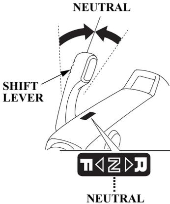
1. Turn the throttle grip to **SLOW** position and move the shift lever to **NEUTRAL**.
