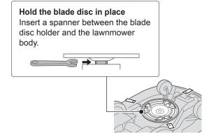
Replace the blades, insert each blade through each bolt on the blade disk, and lightly tighten a nut with the 8 mm spanner.
