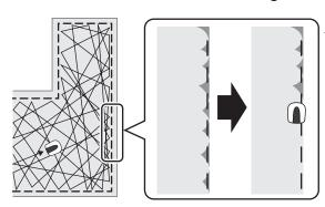
If the edge cutting setting is enabled, the lawnmower goes around your garden along the boundary wire to mow the edge before starting the usual mowing.
