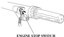
1. Move the shift lever or the control lever to the N (neutral) position and stop the engine.
