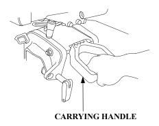
• Do not carry the outboard motor by the carrying handle more than five minutes. Prolonged carrying of the outboard motor by the handle can cause the engine oil leak in the cylinders, make the engine hard starting or smoke when started.
