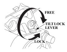
Use the tilt lock lever to raise the outboard motor and lock it in the position when the boat is moored or anchored for a long time.
