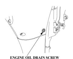
2. Remove the engine oil drain screw and drain the engine oil.
