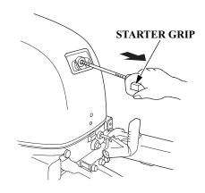
Pulling the starter grip operates the recoil starter to crank the engine for starting. Set the shift lever in the N (neutral) position before starting.
