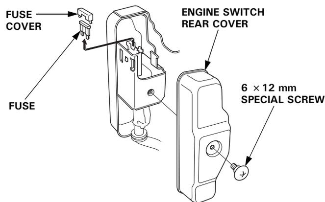
Frequent fuse failure usually indicates a short circuit or an overload in the electrical system. If the fuse burns out frequently, take the engine to a Honda servicing dealer for repair.
