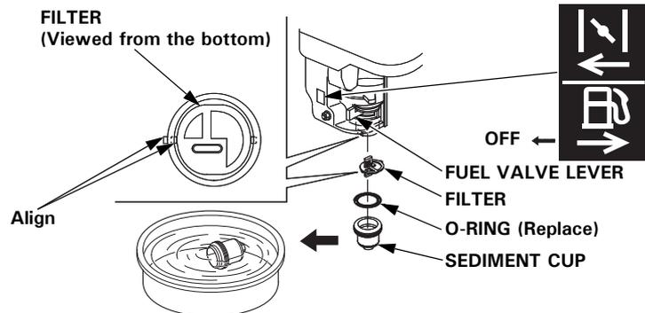
3. Reinstall the filter, new O-ring, and the sediment cup. Tighten the sediment cup securely.
