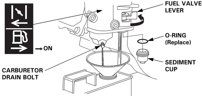
4. After all fuel has drained into the container, tighten the carburetor drain bolt securely.
