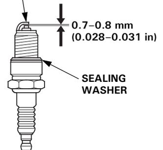
6. After the spark plug is seated, tighten with a 13/16-inch spark plug wrench to compress the sealing washer.
