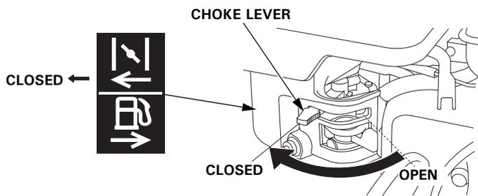
To restart a warm engine, leave the choke lever in the OPEN position.
