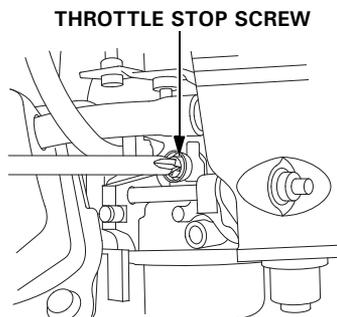
Standard idle speed: 1,400<sup>+200</sup><sub>-150</sub> rpm
