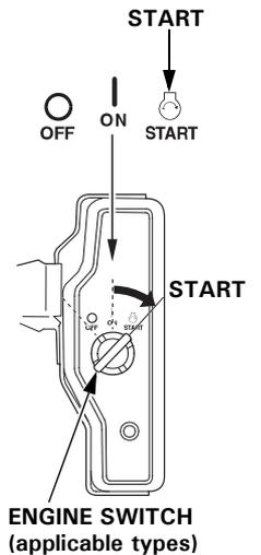
6. If the choke lever was moved to the CLOSED position to start the engine, gradually move it to the OPEN position as the engine warms up.
