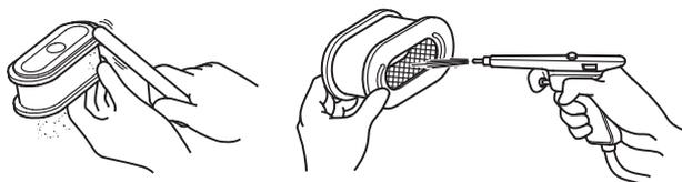
Foam filter element: Clean in warm soapy water, rinse, and allow to dry thoroughly. Or clean in non-flammable solvent and allow to dry. Dip the filter element in clean engine oil, and then squeeze out all excess oil. The engine will smoke when started if too much oil is left in the foam.
