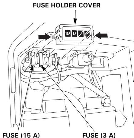
5. Install the fuse holder cover and the battery maintenance cover in the reverse order of removal (see page 51).
