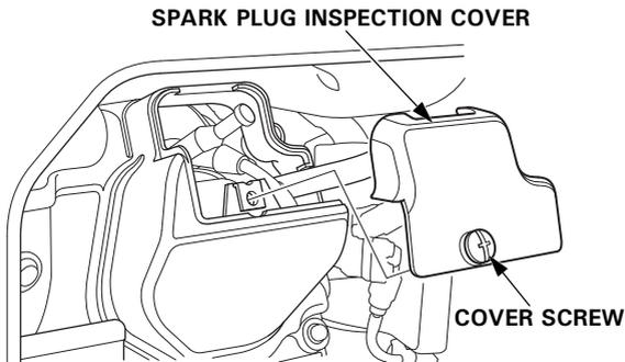
3. Disconnect the spark plug cap, and remove any dirt from around the spark plug area.
