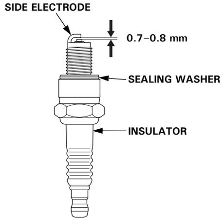
7. Make sure that the spark plug sealing washer is in good condition, and thread the spark plug in by hand to prevent cross-threading.
