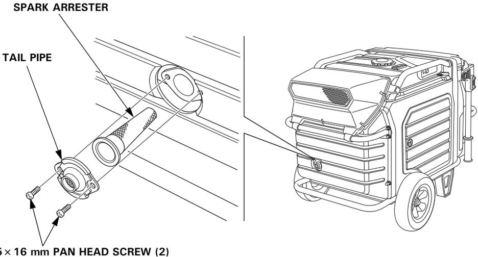
2. Use a brush to remove carbon deposits from the spark arrester screen.
