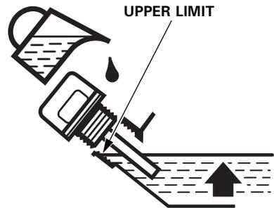
The Oil Alert system will automatically stop the engine before the oil level falls below safe limits. However, to avoid the inconvenience of an unexpected shutdown, check the oil level regularly.
