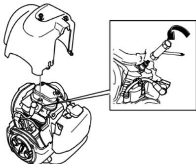
Clean, gap or replace the spark plug.
