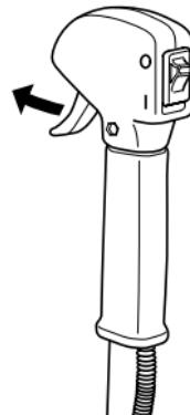
2. Turn the engine switch to the “OFF” position.
