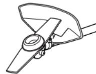
2. Check the blade for crack, nicks, bend and wear. Replace it, if necessary.
