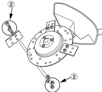
When replacing the blade, change the nuts and washers
