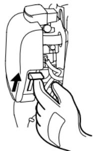
3. Press the priming pump several times until fuel stays in the priming pump.
