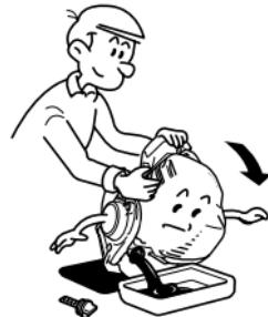
2. Drain the oil by tilting the engine.
