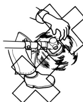
DO NOT TOUCH MUFFLER, WHEN ENGINE IS HOT.
