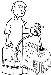
2. Loosen the drain screw and drain the fuel.
