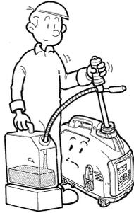
2. Loosen the drain screw and drain the fuel.
