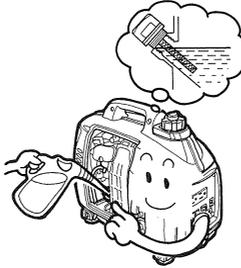
ENGINE OIL CAPACITY: 0.25 L (0.26 US qt, 0.22 Imp qt)
